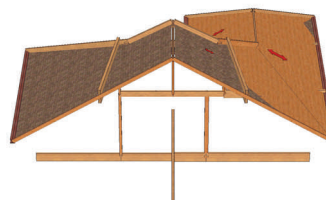
In this roof design, we carried the loads across two floors to keep the open spans below.
